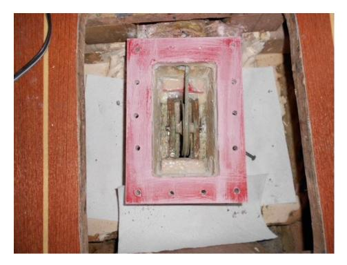
This photo shows the water tight box open with the sheave and cable exposed
