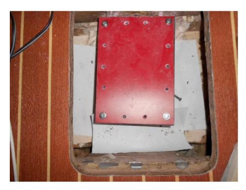
This photo shows the water tight box and lid, lid not bolted in place...this box and cover have been re-built by the owner to allow using a rubber gasket rather than caulking.
